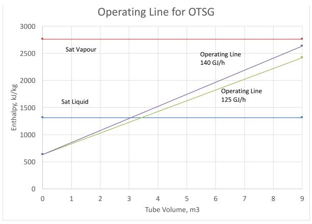
4) Firing rate is increased from 125 GJ/h to 140 GJ/h. What is new steam quality? Show the new operating line and saturation line. What is the new liquid filled volume? How much water mass was gained or lost by the time the OTSG lines out?
